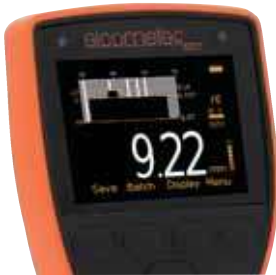
Cross sectional 2D B-Scan, ideal for relative depth analysis.
